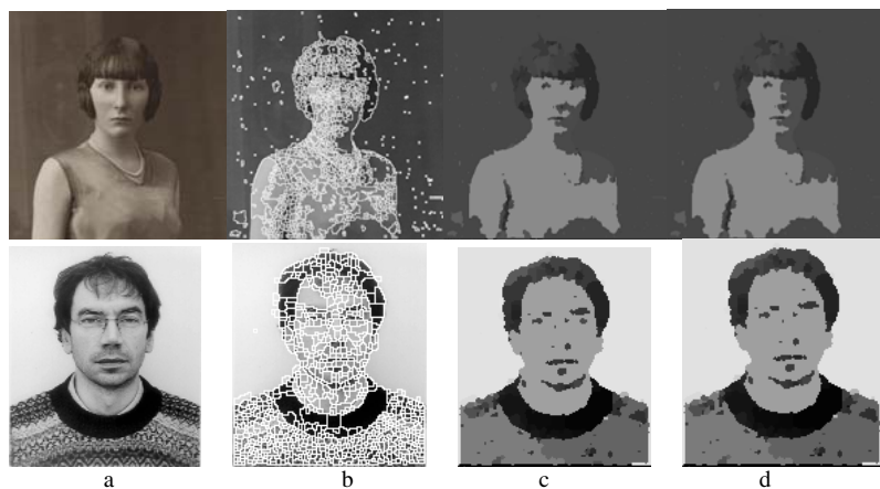
Fig. 7. Original image. b. segmentation obtained with a watershed algorithm. c. final segmentation with the optimal merging threshold d. image obtained with the just higher merging threshold: the semantic graph becomes un-consistent
