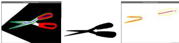
Fig. 8. The points used to compute the model alignment. Left: result of the model-based region grouping, with region group (in green) and matched shock graph (skeleton in blue). Middle: silhouette of model shock graph. Right: those portions (red) of the region group skeleton that match the model shock graph, along with their corresponding contour points (yellow) used to compute the aligning transformation
